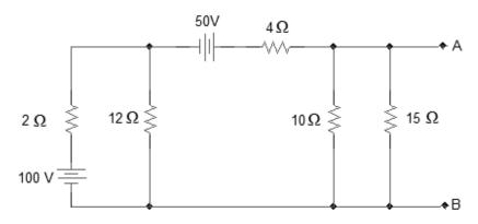
b) Determine the load resistance to receive the maximum power from the source. Also find the maximum power delivered to the load.
